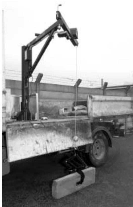
Figure 2 Vehicle-mounted crane and mechanical grab
