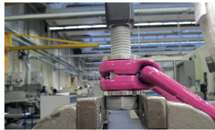
Pic. 8: Dismantling position of the VLBG
