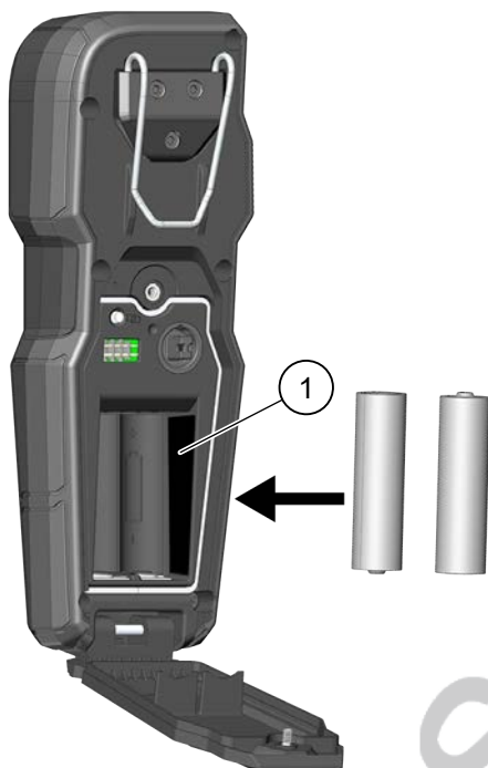
Figure 1. Installing Remote Control Batteries
