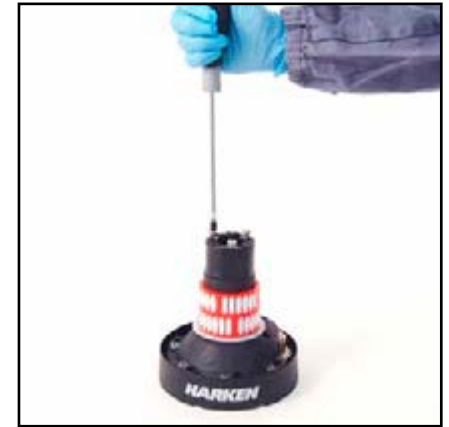
6. Completely unscrew three screws n°27
