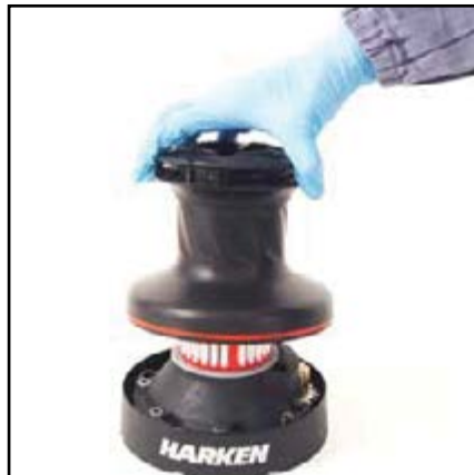
5. Lift off the drum n°22
