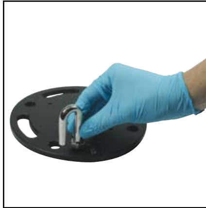
2. Wind rope guide into mounting hole (adjacent to "line in" arrow) as far as possible without it protruding through the plate.
