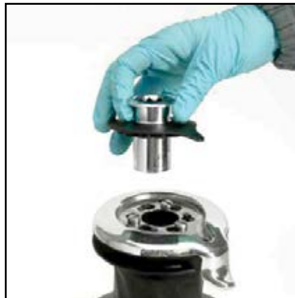
5. Slide off the hub n°20 and the cover n°19
