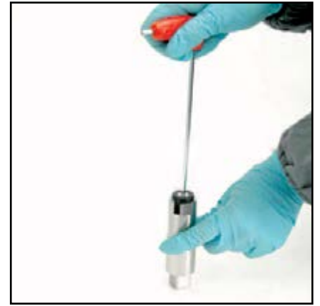
13. Unscrew the screw n°10 and remove the washer n°9. (4 Nm/35 in-lb)
