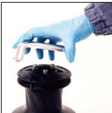
7. Remove the self-tailing arm n°17 by rotating and lifting it.
