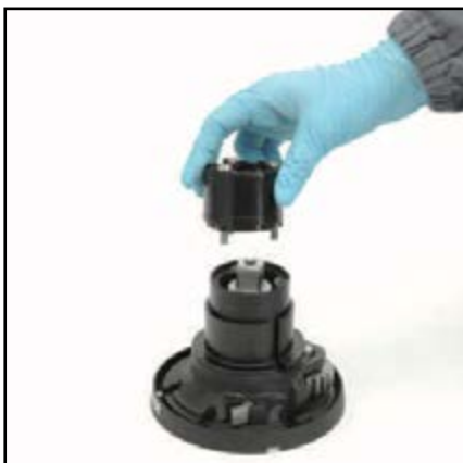
7. Remove the self-tailing arm support n°12 and slide out the bushing
