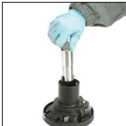
8. Slide out the central shaft n°7
