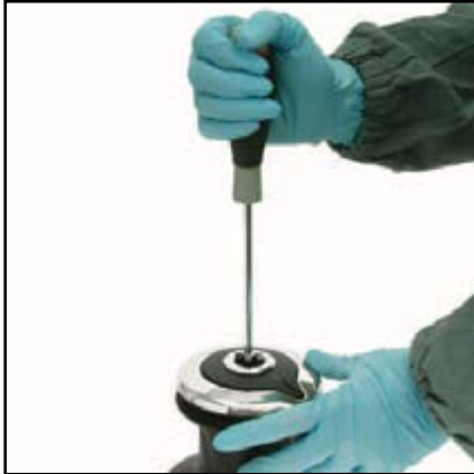
1. Unscrew the central screw ( 2 Nm/18 in-lb)
