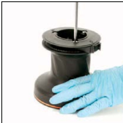
1. Unscrew the 3 screws n°16 ( \approx 4 Nm/35 in-lb)
