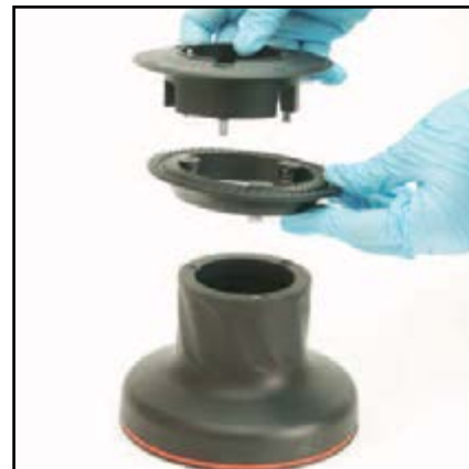
If jaws have been disassembled, insert peeler between two jaws, taking care that letters "TOP" on peeler are facing upwards.
