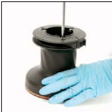
When positioning stripper arm, align peeler with it.
