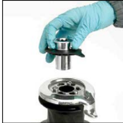
2. Slide off the hub n°20 and the cover n°19
