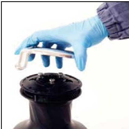
4. Remove the self-tailing arm n°18 by rotating and lifting it.
