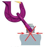
Fig. 5: The lifting point must have been fully bolted in.
