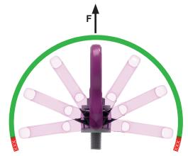
Fig. 8: Pivoting area (green = permitted loading direction)
