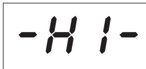
When the load applied to the sensor exceeds the maximum capacity of 10% of device (e.g. a 1 t loaded at 1.1 t) the display unit indicates an overload status message “– HI –” as shown opposite.
