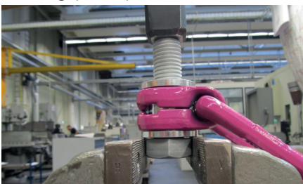
Pic. 8: Dismantling position of the VLBG-PLUS
