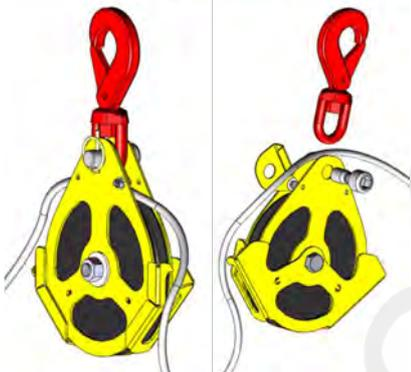
3. Fit the cable inside the carter through the opening. (This operation can also be done before re-installing the axis)
