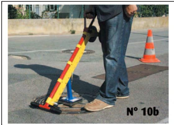
Always position magnet on a plate while controlling LIFTPAQ® by the handle-bars.
