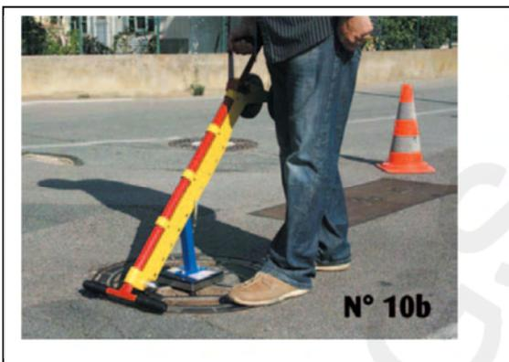
b. **Detaching magnet in an easier way: using retracted handle.** To separate magnet from plate, pull handle back fully, use LIFTPLAQ lifting handle or body to pull up until the magnet is detached. During this operation, instrument handles will be pushing on the ground.
