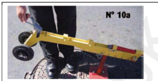
**b. Detaching magnet in an easier way: using handle-bar shaft in retracted position.**
