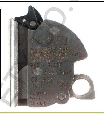
The RGA11 is designed to provide vertical fall protection to operative ascending /descending a ladder or structure. This version of the rope grab is for use with **8mm Stainless Steel Wire Rope Only**. When used by itself, the RGA11 should be connected directly to the chest attachment of a harness (RGH2/RGH4) via a karabiner. This ensures that the operative is held close to the structure and in the event of a slip, the fall distance and loading on the top anchor is minimal.
