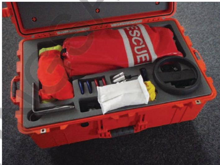
If a relative humidity of more than 50 % is reached, the desiccant bags have to be replaced after checking the case's contents.
