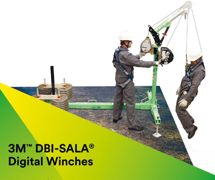
3M<sup>™</sup> DBI-SALA® Digital winches are rated for a maximum working load of 204 kg (450 lbs) with an 11:1 safety factor. This winch has two cranking speeds capable of retrieval/descent from 4 m/min (13 ft/min) to 9 m/min (30 ft/min).
