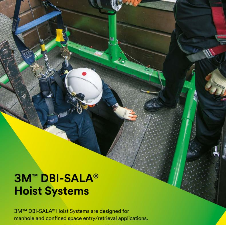
These units are constructed of lightweight materials including high-strength aluminium. The davit pivots for ease-of-rescue and has adjustment for overhead clearance restrictions. The lower base adjusts to fit most standard entries. Many other portable and fixed bases are available to suit any jobsite need.
