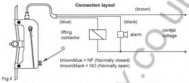
The switching power is 4 A, 220 Vac (0.3 A, 250 Vdc). (It is therefore possible to connect in series in the upper limit switch circuit.)
