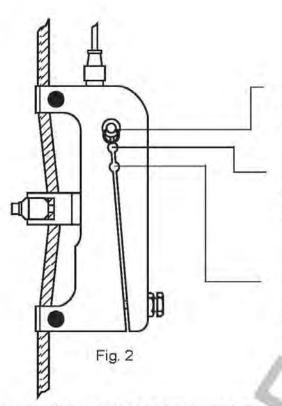
For wire rope 17 mm diameter and for loads ranging from 300 kg to 2500 kg without the rubber compression pad.
