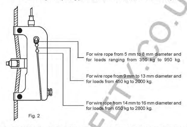
Correct positioning of the tightening bracket depending on the diameter of the wire rope.
