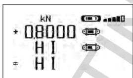
If several sensors are connected to the display unit, the overloaded sensor will be immediately identified. In the example display opposite, relating to a two-sensor set up, the sensor on the second line is overloaded.
