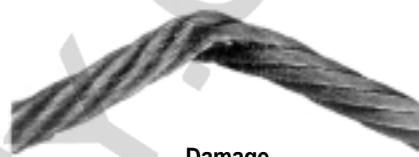
Damage caused by improper use, (e.g. by fixing the load with the rope)
