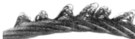
Loop formation on wire rope
