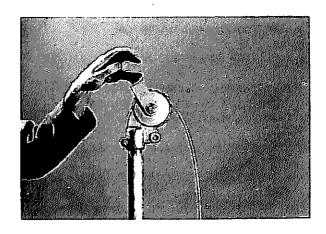
When used on a Tripod the tube mounted enclosed drum Hoist can be attached to a mounting bracket that fixes to one of the legs.
