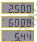
Display of rated load with unit of measure (e.g. 2.500 t)
