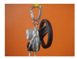
The handwheel can be rotated to elevate the accident victim till he/she can either be lifted to a secure base or the securing lanyard of the person to be rescued can be detached. When doing so, the slack rope between the turning device and the cam cleat is pulled downward and tightened over over again. This helps minimising the distance over which the person to be rescued may slip in case the handwheel is inadvertently released.
