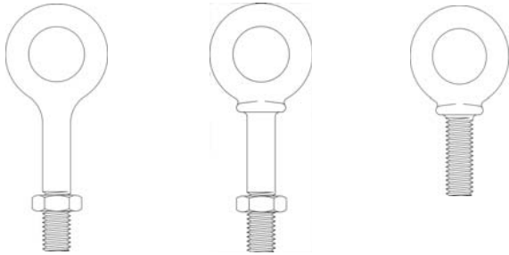
Regular Nut Eye Bolt G-291 Shoulder Nut Eye Bolt G-277 Machinery Eye Bolt S-279 / M-279
