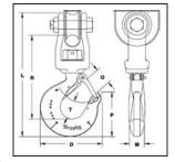
Suitable for infrequent, non continuous rotation under load.
