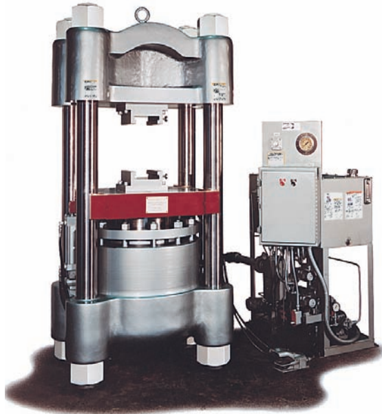
1500 Ton Hydraulic Swaging Machines Approximate weight 34,500 lbs. Overall height 8 ft. 6 in. Fast advance and retract speed. Automatic slow, precision swaging speed.
