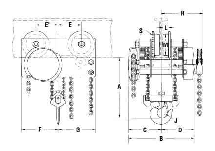
Beam profile and dimension as well as curve radius must always be specified when ordering.
