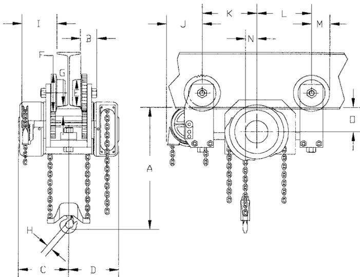
**Beam profile and dimension as well as curve radius must always be specified when ordering.**
