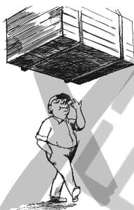
After lifting or tensioning, a load must not be left unattended or remain lifted for a longer period of time.
