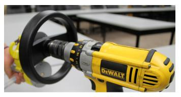
Protruding 10 mm diameter shaft on the hub is used as a drill adaptor. Connect the Power Drill to help control the pace and / or raise the fall victim. Min advised torque : 45 N.m. Min rotating speed : 0-300 turns/min
