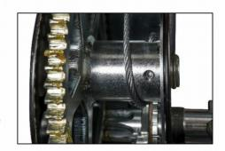
The protective cover can be reassembled again by means of the four M6 hexagon screws.
