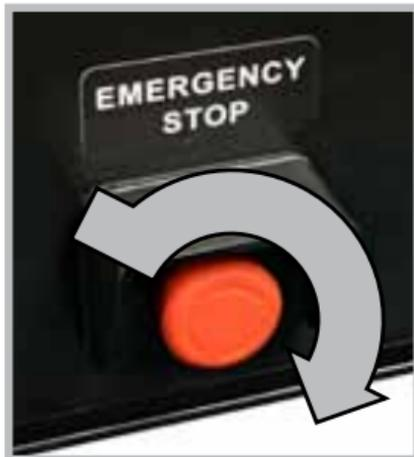
There is also an emergency stop button on the base unit. Push in to activate and twist clockwise to release
