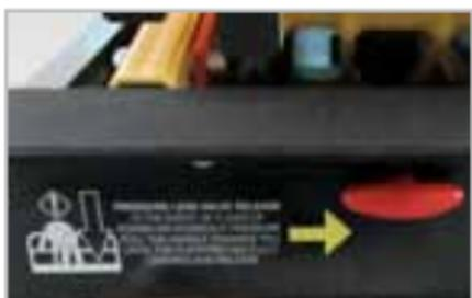
Emergency pressure loss valve release handle
