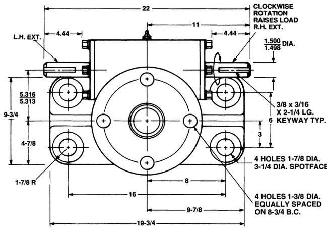
4 1/2" Diameter x .666 Lead Lifting Screws
