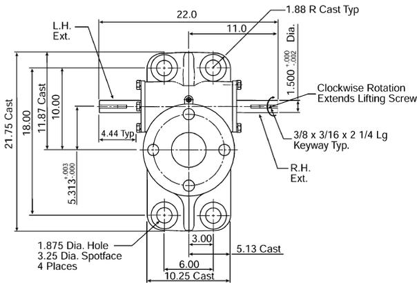
4 1/2 Diameter x .666 Lead Lifting Screw
