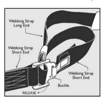
connectors may be fitted conforming to EN362). This lanyard is only for use with the EN358 Work Positioning 'D' rings fitted to a suitable P&P harness. It then serves to provide a hands free environment. The Webbing Strap can be increased
