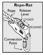
The 'Rope-Rat' attachment point is normally supplied with a screwed oval link but may be fitted with a self closing/self locking EN362 connector. The free end of the rope is 'sewn back' to prevent the 'Rope-Rat' detaching from the rope end.
