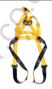
The RGH5 is designed for use as a confined access harness. The front and rear attachment points can be used as standard fall arrest points and the rescue strap can be used for lifting and lowering. When used, the rescue strap keeps the operative in a near vertical position, which is preferred when recovering an unconscious casualty.
