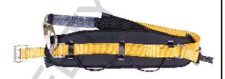
The **RGB180BT** is a work positioning belt. This belt is fitted with an integral work positioning strap that can be passed around a pole or similar structure and clipped back onto the remaining side D ring. The Work Positioning strap is fully adjustable and is fitted with an anti abrasion wear pad and double action safety snap hook.
