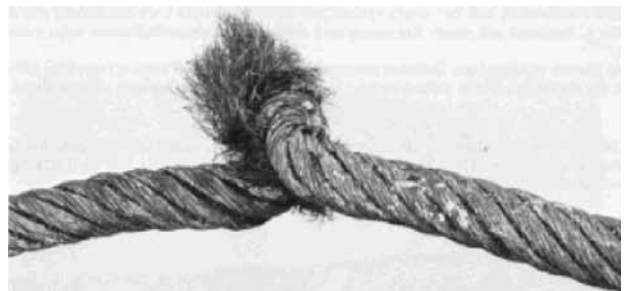
Figure 5: Wire rope with kink
