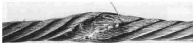
Figure 4: Wire rope with flattening caused by being run over
