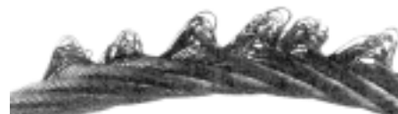
Loop formation on wire rope
