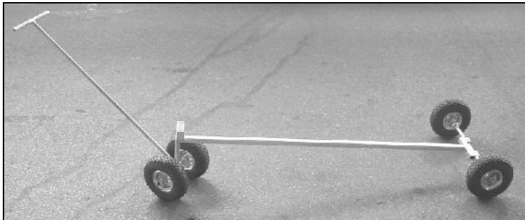
Picture 4.3 Pulling carriage for the components Gantry Crane FAG-3222-2M
