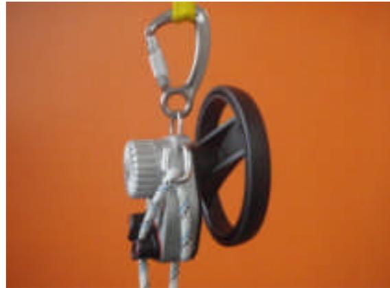
The handwheel can be rotated to elevate the accident victim till he/she can either be lifted to a secure base or the securing lanyard of the person to be rescued can be detached. When doing so, the slack rope between the turning device and the cam cleat is pulled downward and tightened over and over again. This helps in minimising the distance over which the person to be rescued may slip in case the handwheel is inadvertently released.
