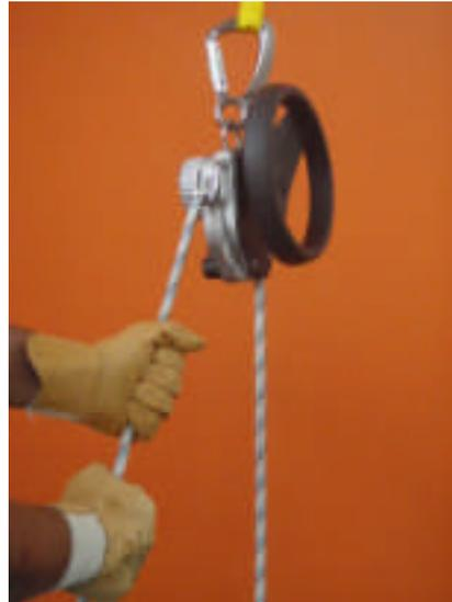
The movement velocity is automatically controlled via a centrifugal brake. In addition, the person on the base (the rescuing person) also has the option of holding onto the rope in his/her hands, thus stopping the descent.
