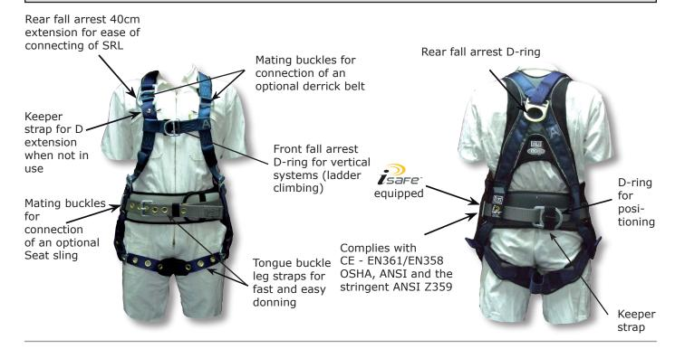
**Especially designed** for the oil extraction worker. It includes connection for optional derrick belt which provides the worker with restraint and comfort with the large frontal pad while positioning for the next drilling pipe. Alternatively on the rear of the harnesses belt there is a D connection point.
