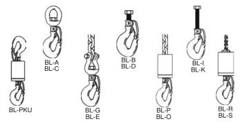
QUIC-CHECK® Hoist Hooks incorporate markings forged into the product which address two (2) QUIC-CHECK® features: Deformation Indicators - Two strategically placed marks, one just below the shank or eye and the other on the hook tip, which allows for a QUIC-CHECK® measurement to determine if the throat opening has changed, thus indicating abuse or overload.
