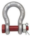
G-2130 / S-2130 Bolt Type Anchor shackles with thin head bolt - nut with cotter pin. Meets the performance requirements of Federal Specification RR-C-271F Type IVA, Grade A, Class 3, except for those provisions required of the contractor. For additional information, see page 475.
