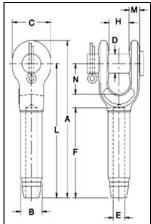
NOTE: S-501 Swage Sockets are recommended for use with 6 x 19 or 6 x 37, IPS or XIP (EIP), XXIP (EEIP), RRL, FC or IWRC wire rope. Before using any National Swage fitting with any other type lay, construction or grade of wire rope, it is recommended that the termination be destructive tested and documented to prove the adequacy of the assembly to be manufactured. In accordance with ASME B30.9, all slings terminated with swage sockets shall be proof loaded.\*
