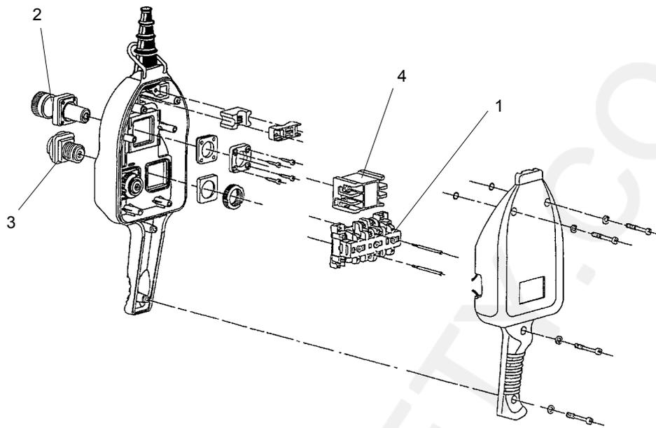
**Fig. 25: Pendant switch for contactor control**
