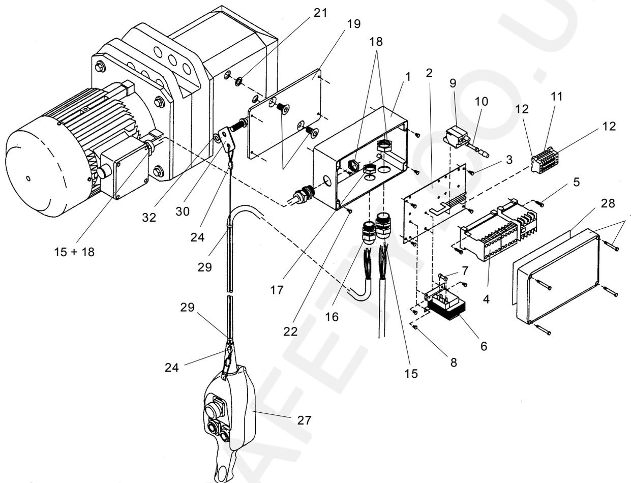
Fig. 22: Contactor control
