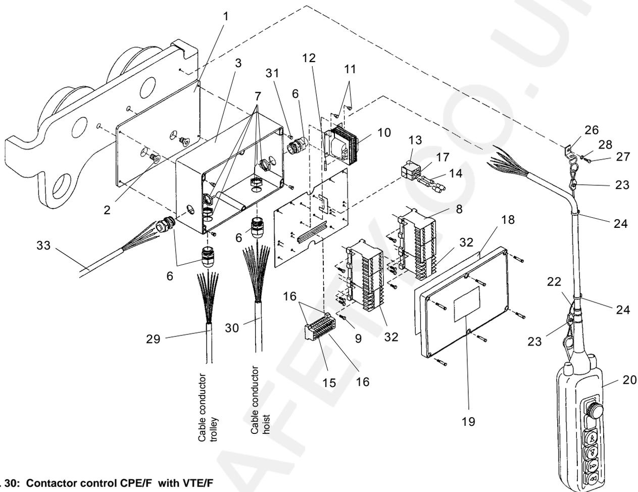
Fig. 30: Contactor control CPE/F with VTE/F
