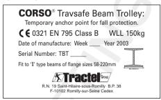
Travsafe trolleys should only be used with a maximum load equal to the nominal load shown on the name plate.
