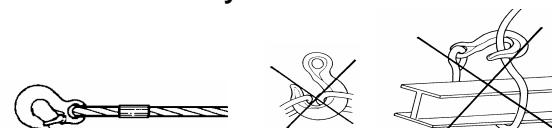
**do not use the winch rope as a hitching device**
