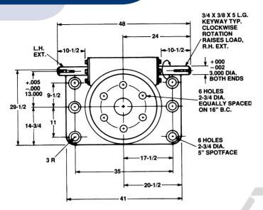
9" Diameter x 1" Lead Lifting Screws
