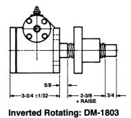
Note: Lifting screw is not keyed. Top should be secured to a lifting member to prevent rotation. When a Bellows Boot is required, see pages 143-144. Dimensions are subject to change without notice.
