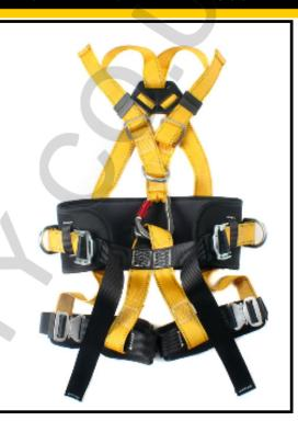
The RGH16 is a further innovation of the Ridgegear range of safety harness. For fall arrest the harness comprises front and rear D rings. In addition there is the added benefit of 2 side D work positioning D rings on a comfortable support pad, and a further ventral front D ring positioned at the waist for sit suspension and / or work positioning.
