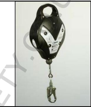
A lighter weight and smaller block than the RGA2, the RGA26 is also a multi purpose fall arrest block, which allows uninhibited movement during normal working activity. The carrying handle is part of the cast alloy housing and can be connected to the anchorage point using soft slings or a karabiner.
