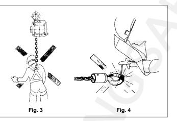
• Avoid side pull, i.e. side load on either housing or bottom block (Fig. 5). Lift only when the load chain froms a straight line between both hooks.
