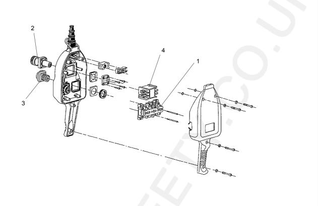
Fig. 25: Pendant switch for contactor control
